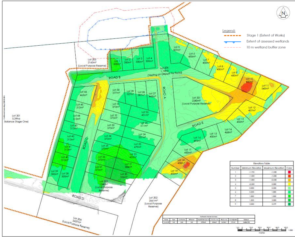
Figure 2: Extent of work for Stage 1. Source: Engineering Service Report – Proposed Cuts & Fills Plan.
