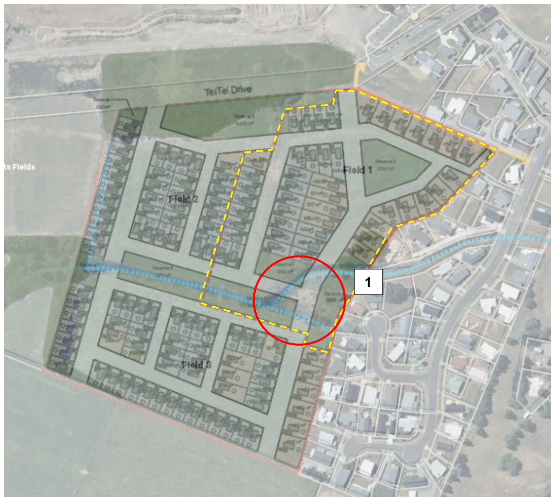
Figure 15 - Site development overlay with current site conditions underneath, red circles denote areas that will need detailed planning to address effects on streams. Stage 1 shown as yellow dashed line.
