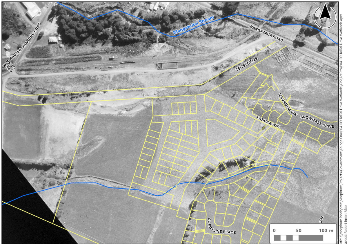
Figure 9: Aerial image of the site from 1963 showing railway to the north and earthworks into the north west of the site.
